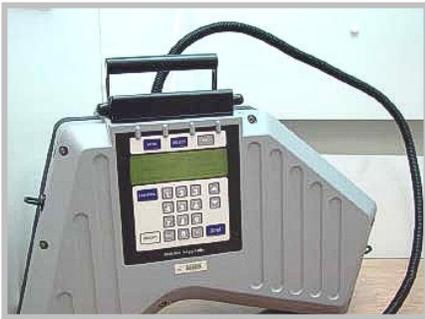
**Figure 2:** Photograph of the Miran SaphiRe Infrared Analyzer Model 205A
